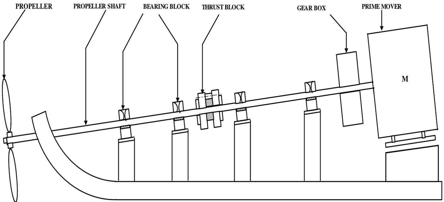
**2.2.4.2F-** A schematic diagram of a typical marine propulsion shafting
