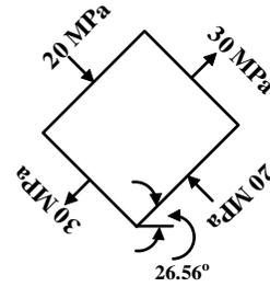
**2.2.6.2F-** Orientation of the loaded element in the left to show the principal stresses.
